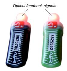
SIAC contains a battery and will always work in direct punching mode even if the battery is empty. Direct punching provides a fall-back option to register at controls. In contactless punching mode the SIAC's optical and acoustic feedback signals confirm that a control code and timestamp have been successfully written to the card.
