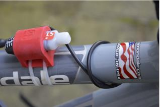
**WRONG** - Battery leads shall NOT be positioned by the SIAC
